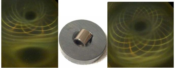
Below: Image on left, two cylinder magnets on the right connected along their non-polarized sides. Image on right broken ring magnet.
