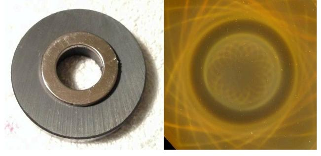
Below: Two color inverted images of ring magnets under the ferrocell. Notice the perfect pair of inner and outer hypotrochoid of convergence and divergence.
