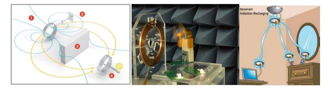
Below and above: New developments in wireless recharging technology are being developed that will allow the charging of multiple devices at the same time without needing wires using magnetic resonance (right illustration). On the left, another company is using antennas to beam form electromagnetic energy to remote devices up to 15 feet. The powered wireless router tracks the devices and beam forms the electromagnetic energy to the device to charge it.
