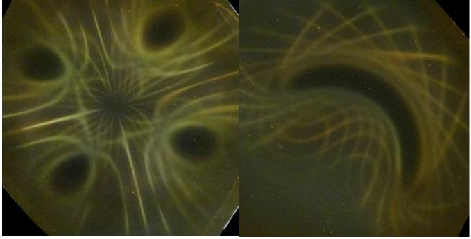
Below: ½" cylinder magnet along one pole on the left, and two of the same cylinder magnets on the right connected along their non-polarized sides. Notice the voidance pattern in the middle between these four poles.
