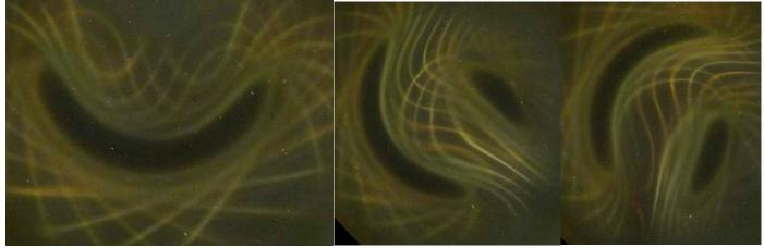
Below: Large ceramic magnet with neodymium magnet attached. On right showing both together under the ferrocell. With field pressures equalized both magnets appear no different than a single ring magnet.
